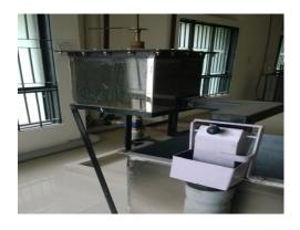
The purpose of this experiment is to demonstrate and verify the integral momentum equation. The force generated by a jet of water detected by an impact surface is measured and compared to the momentum change of the jet.
