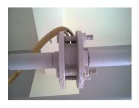
Measurement of the flow rates of liquids, gases and vapors with orifice meters has found wide use both in industrial and in scientific measurements. It consists of a flat orifice plate with a circular hole drilled on it. There is a pressure drop between upstream from the orifice plate and just downstream from which the flowrate can be deduced which gives a measure of the discharge.
