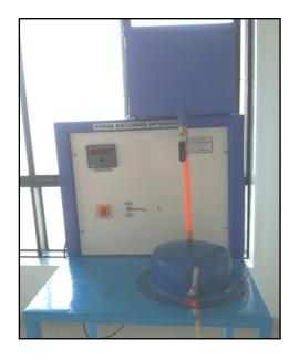
A copper test disc is fitted at the center of jacket. The hot water is obtained from a hot water tank, fitted to the panel, in which water is heated by an electric immersion heater. The test disc is then inserted at the center with thermocouple. Thermocouples are fitted inside hemisphere to average out hemisphere temperature. A timer with a small buzzer is provided to note down the disc temperatures at the time intervals of 5 seconds.
