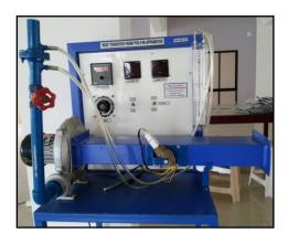
Extended surfaces or fins are used to increase the heat transfer rates from a surface to the surrounding fluid wherever it is not possible to increase the value of the surface heat transfer coefficient or the temperature difference between the surface and the fluid.
