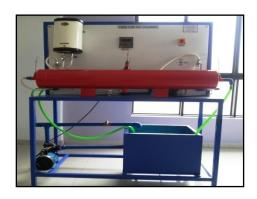
In this type of heat exchanger, fluids move usually perpendicular to each other and such flow configuration is known as cross flow heat exchanger. In compact heat exchangers, cross flow arrangement is used. It is further classified in two ways: mixed and unmixed cross flow heat exchanger.
