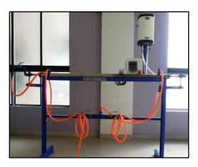
The simplest type of heat exchanger consists of two concentric pipes of different diameters known as double pipe heat exchanger. In parallel, both hot and cold fluids enter the heat exchanger at the same end and move in the same direction. In Counter flow, on the other hand, hot and cold fluids enter the heat exchanger at the opposite end and move in the opposite direction.
