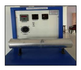
The most important characteristics of any insulation material include a low thermal conductivity, low tendency toward absorbing water, and of course the material should be inexpensive. With the help of this setup; can understand the perfect insulation thickness in terms of radial thickness.
