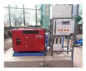
The setup consists of single cylinder, four stroke, VCR (Variable Compression Ratio) kerosene engine connected to AC/DC type dynamometer for loading. The compression ratio can be changed without stopping the engine and without altering the combustion chamber geometry by specially designed screw on cylinder block arrangement. The setup enables study of VCR engine performance parameter like BP, IP and heat balance sheet.
