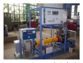
variable load on engine to study engine performance under variable load conditions. Exhaust gas calorimeter is used for estimation of heat carried away by exhaust gases for determination of heat balance of the engine. Air is supplied to the engine through an air box, fitted with orifice plate. The instrumentation console includes measuring instruments for engine speed, fuel consumption & temperature of water, gases.
