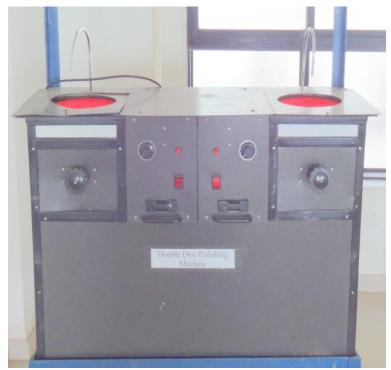
It is used for dry or wet polishing of the specimen whom metal structure to be observed.
