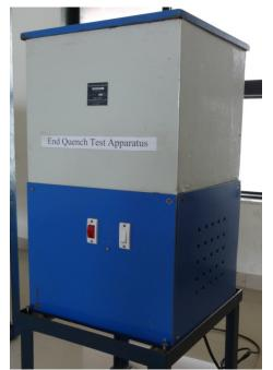
This apparatus is used to know the effect of quenching medium on hardness of steel.
