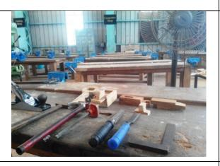
Carpentry may be designed as the process of making wooden articles and component. Carpentry involves cutting, shaping and fastening wood and other materials together to produce a finished product. Various types of Marking and Measuring tools (Marking gauge, Try square), Holding tools (Carpenter's vice), Planing tools (Jack plane), Cutting tools (Saw, Chisels) are used in carpentry shop.
