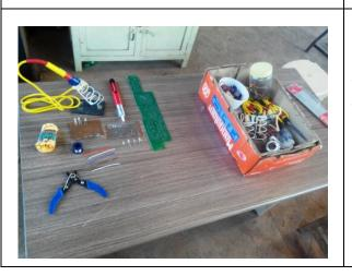
**Soldering** is the process in which two or more metal items are joined together by melting and flowing a filler metal (solder) into the joint. The tools like Soldering lead, Soldering Iron, Tester, Solder Cleaner and Clipper are used in Soldering shop. Soldering is used in electronics (for PCBs) and metalwork from flashing to jewelry.
