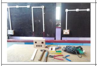
**Electrical shop** gives an exposure to student for basic electric devices and fittings as well as intricacies involved in domestic and industrial electrical wiring. Practical's like identification of phase, neutral and earth of domestic appliances and their connection to two pin/three pin plugs are performed by the students.
