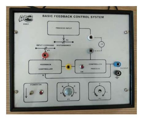
This kit demonstrates the principle and working of a Basic Feed control system with input supply of 230V, 50Hz AC.
