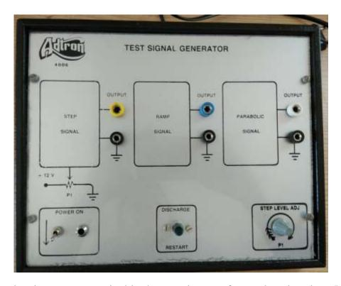
It is a complete instrument, required in the experiments of control engineering. It provides test signals of different waveforms and frequencies for feeding in as error signals. The input supply required is 230V, 50Hz AC. It gives very low frequencies (variable) step and Ramp waveform signals, which are essential for finding the response of various control circuits.
