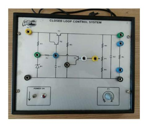
This kit demonstrates the principle & working of Closed Loop Control System and also has provision to connect/disconnect the load & feedback loop and vary the output voltage. The input supply to the kit is 230V, 50Hz AC.Multi – coloured test points are provided at various stages in the circuit to observe the waveforms & voltages.
