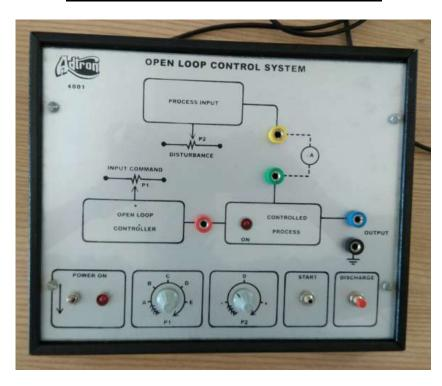
This Kit demonstrates the principle and working of a basic open loop control system and it requires 230V, 50Hz AC supply. It consist of IC based DC regulated power supply with short circuit protection and LED indication for supply "ON". It has in-built variable input command, variable disturbing / error signal and timer with relay.Multi – coloured test points are provided at various stages in the circuit to observe the voltage and waveform.
