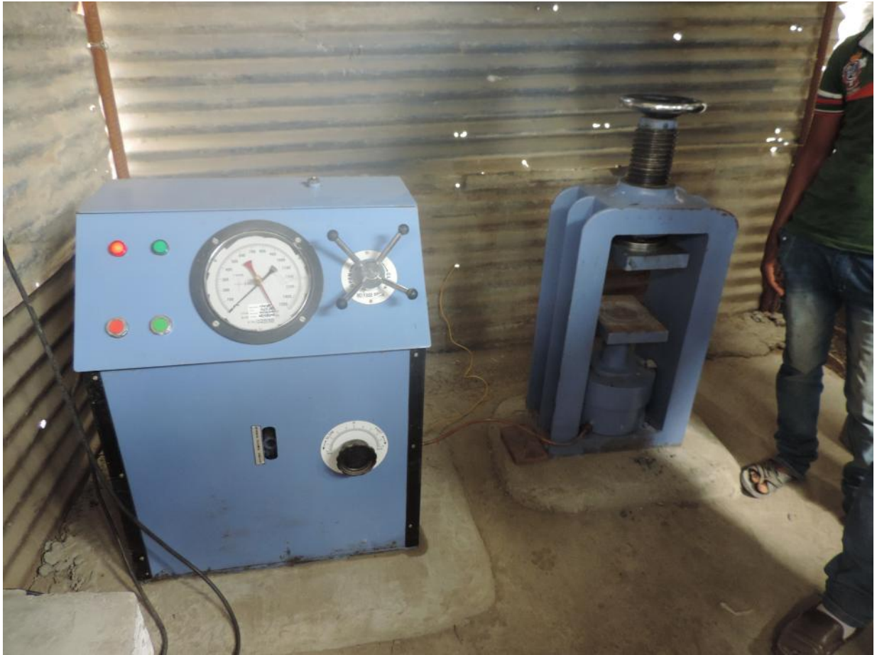
Compression testing machine (Cube Testing)
