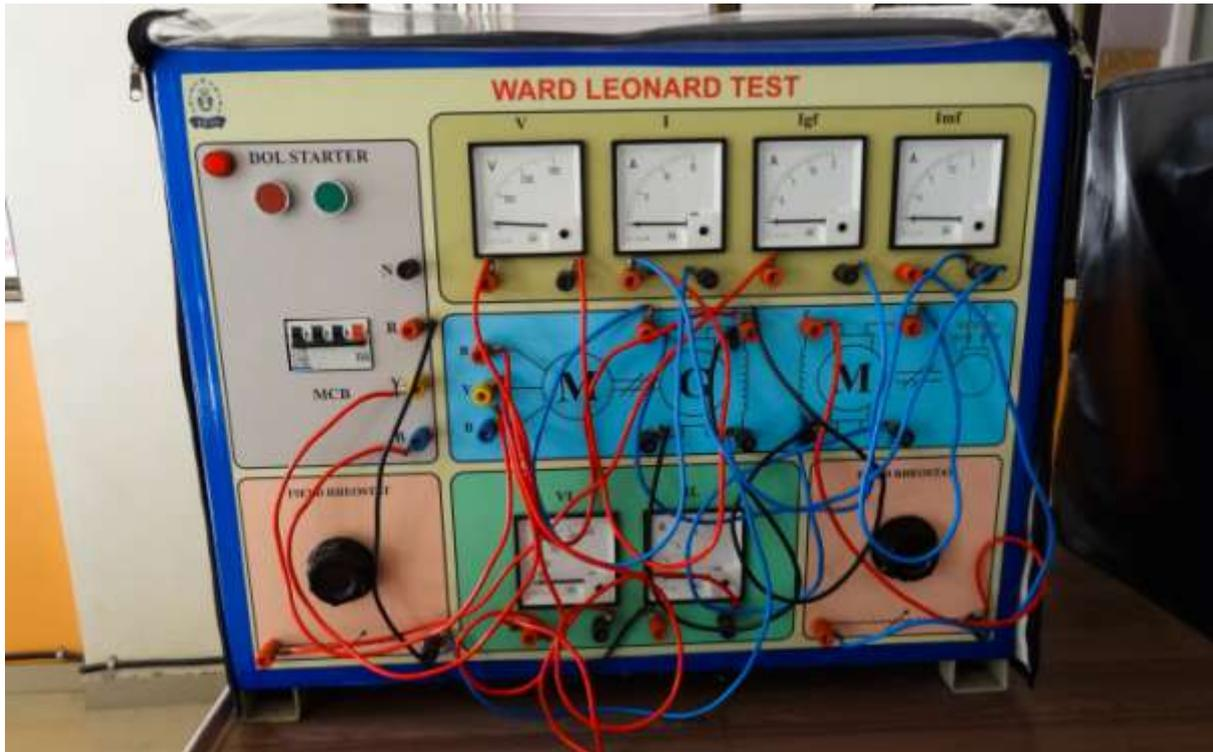
This is essentially armature voltage control of speed with constant field excitation. In this method the variable voltage to be applied to the motor armature is obtained from an additional separately excited d.c generator, and the motor under control is also run as a separately excited motor. The above equation shows that if the motor excitation is constant and the applied voltage  $V$  is varied the speed will be almost directly proportional to the armature voltage.
