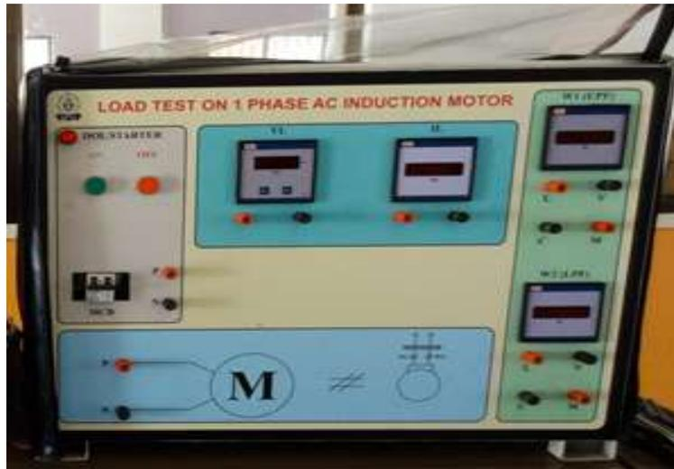
The **load test** on induction motor is performed to compute its complete performance i.e. torque, slip, efficiency, power factor etc. During this test, the motor is operated at rated voltage and frequency and normally loaded mechanically by brake and pulley arrangement from the observed data, the performance can be calculated using suitable equations.
