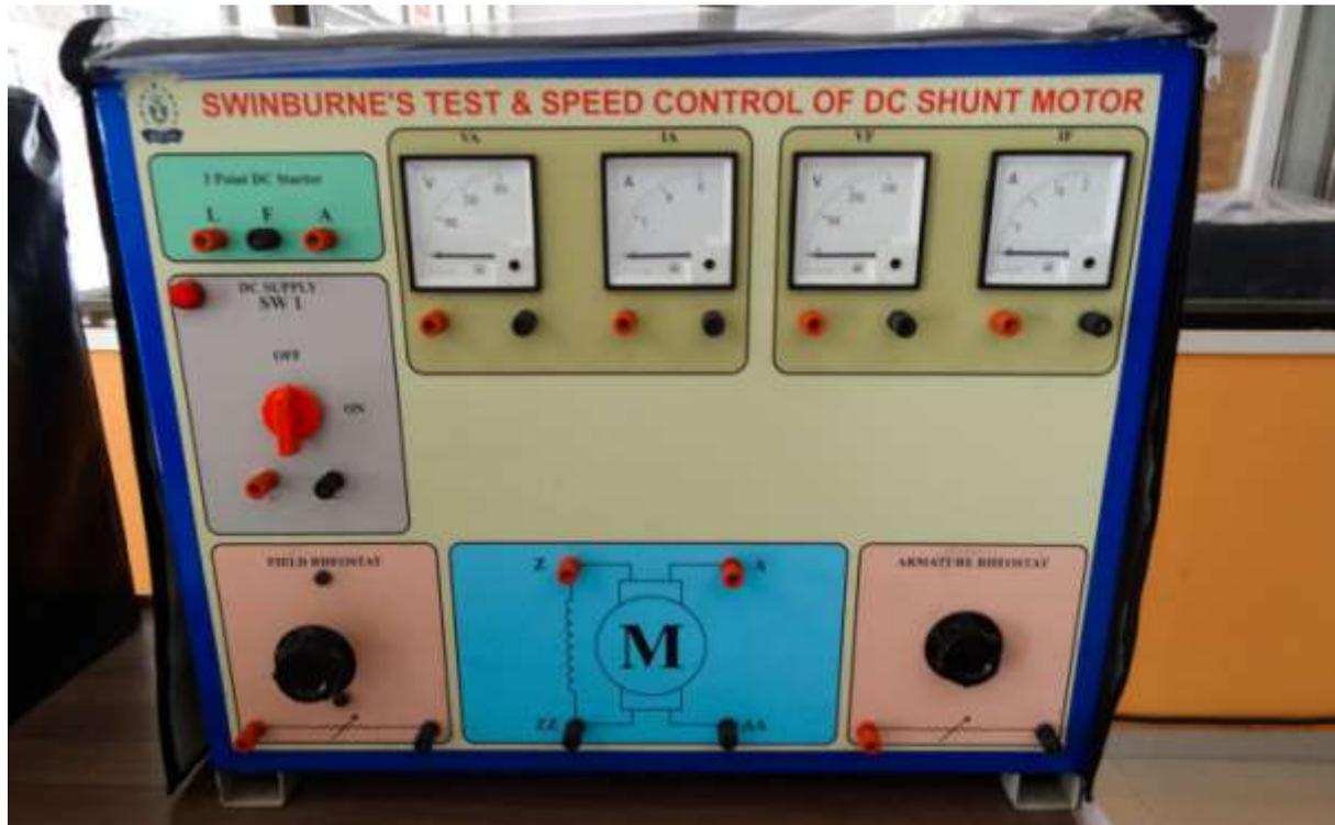
Swinburne's test is the simplest **indirect** method of testing dc machines. In this method, the **dc machine**(generator or motor) is run as a motor at no-load and losses of the machine are determined. Once the losses of the machine are known, its efficiency at any desired load can be determined in advance.
