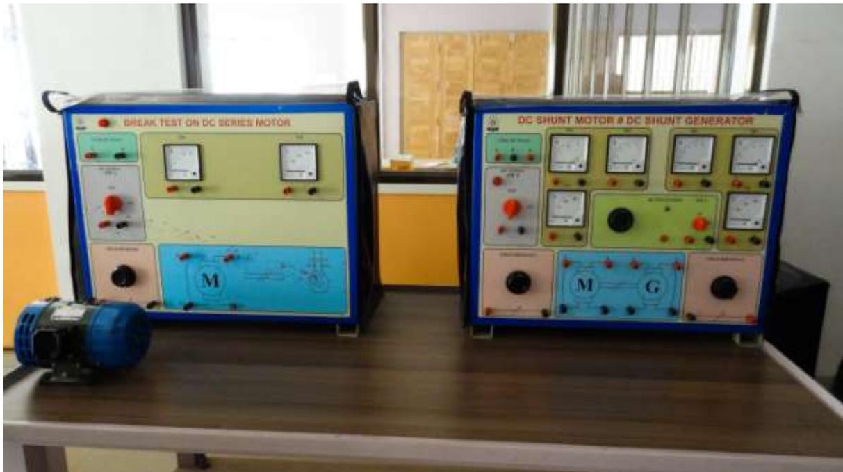
To obtain the performance characteristics of a DC shunt motor by load test.
