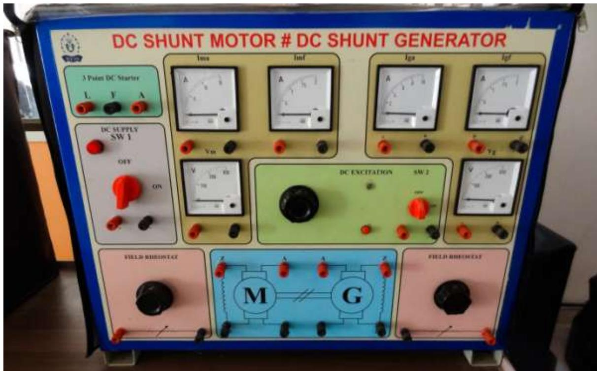
A DC motor takes electrical energy and converts into mechanical energy whereas a DC generator converts mechanical energy into electrical energy. When used as a motor the inputs are Armature Voltage ( $V_a$ ) and Mechanical Load Torque ( $T_{me}$ ).
