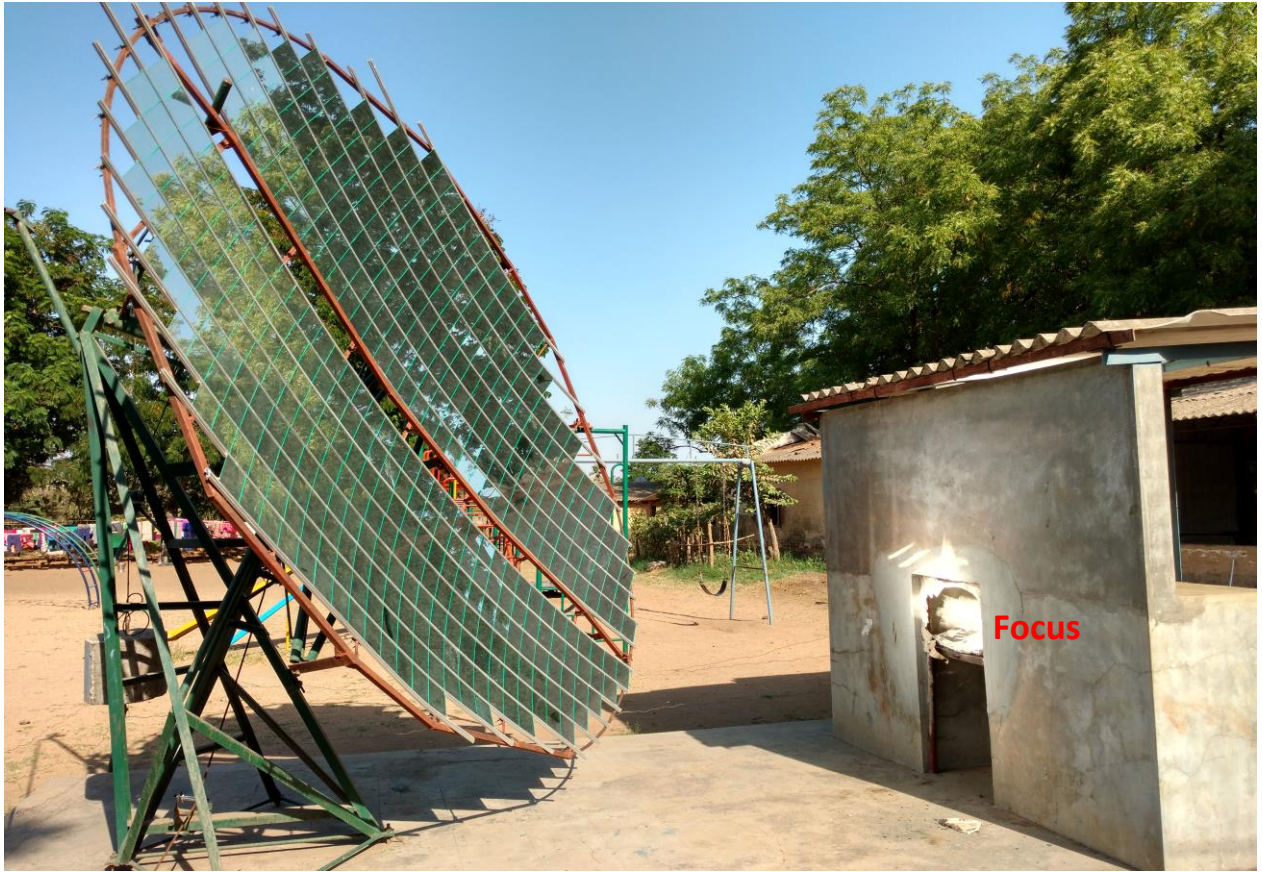
SK 14 Solar Collector Dish at School for Cooking
