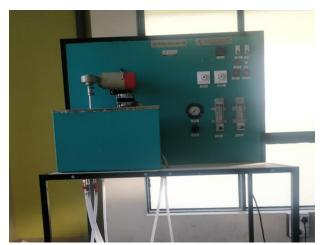
temperature of bath can be maintained from ambient to 90° C with the help of digital Temperature indicator cum controller. Sample can be taken out with the help of a sampling pipette.
