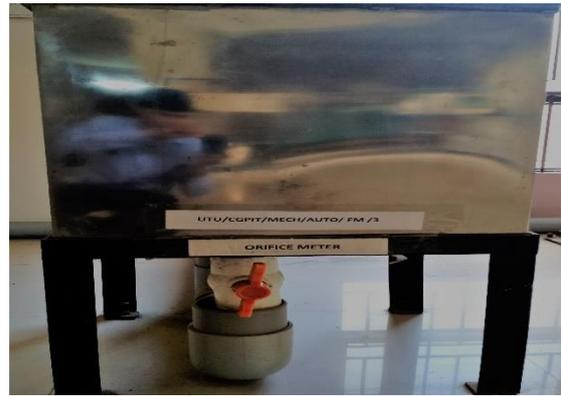
The basic principle on which a orifice meter works is that by reducing the cross-sectional area of the flow passage, the fluid is accelerated and a pressure different is developed, and measurement of the pressure different (between inlet of the meter and a point of reduced pressure) enables the determination of the discharge flow rate through the pipe
