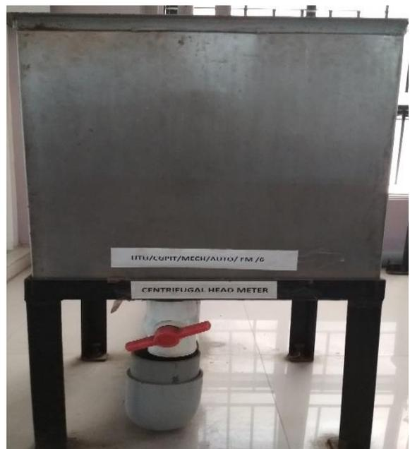
Centrifugal head meter can be used only when the velocity of flow in pipe line is rather high as the differential pressure caused by the primary element is rather
