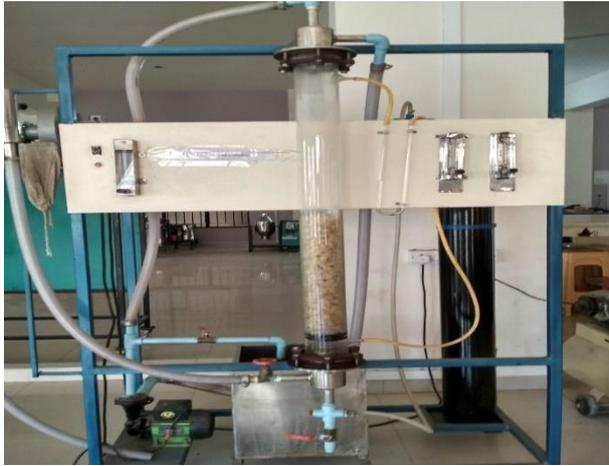
Chemical Engineering operations commonly involve the use of packed beds. These are devices in which a large surface area of contact between a liquid and a gas, or a solid and a gas or liquid is obtained for achieving rapid mass and heat transfer and for chemical reactions. From a fluid mechanical perspective, it is used to determine the pressure drop per unit length of bed
