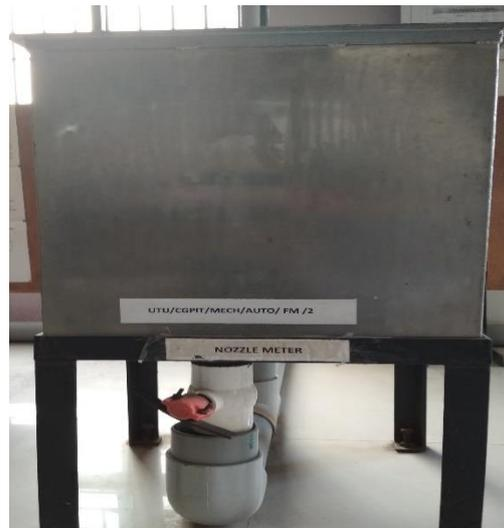
The flow nozzle meter is simple in construction and is less costly in comparison with the Venturi meter though it is capable of handling the same discharge as the Venturi meter.
