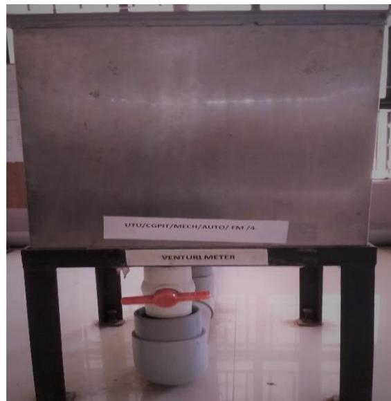
The basic principle on which venturi meter works is that by reducing the cross - sectional area of the flow passage, a pressure difference is created and the measurement of the pressure difference enables the estimation of the discharge/flow rate through the pipe
