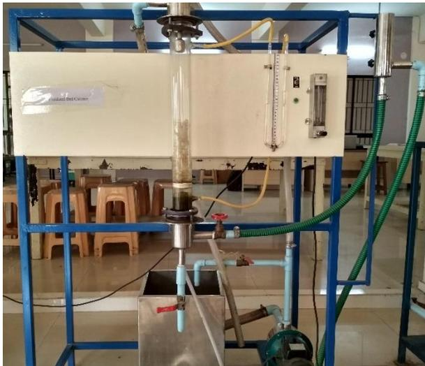
Fluidization of a particle bed, it is necessary to determine what range of flow rates allow fluidization, and also, what flow rates will begin to carry the particles out the top of the particle chamber. Extensive use of fluidization in petrochemical industry with the development of fluid catalytic cracking
