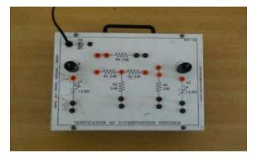
Superposition Theorem Stated as: In a network of linear resistances containing more than one generator (or source of e.m.f), the current which flows at any point is the sum of all the currents which would flow at that point if each generator where considered separately and all the other generators replaced for the time being by resistances equal to their internal resistances.
