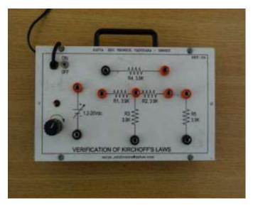
KCL:"At any node (junction) in an electrical circuit, the sum of currents flowing into that node is equal to the sum of currents flowing out of that node, or: The algebraic sum of currents in a network of conductors meeting at a point is zero". The sum of currents entering the junction is thus equal to the sum of currents leaving. This implies that the current is conserved (no loss of current).
