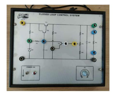
This kit demonstrates the principle & working of Closed Loop Control System and also has provision to connect/disconnect the load & feedback loop and vary the output voltage. The input supply to the kit is 230V, 50Hz AC.Multi – coloured test points are provided at various stages in the circuit to observe the waveforms & voltages.
