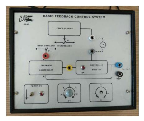
This kit demonstrates the principle and working of a Basic Feed control system with input supply of 230V, 50Hz AC.
