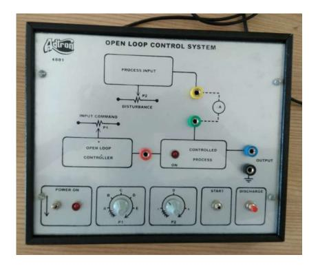
This Kit demonstrates the principle and working of a basic open loop control system and it requires 230V, 50Hz AC supply. It consist of IC based DC regulated power supply with short circuit protection and LED indication for supply "ON". It has in-built variable input command, variable disturbing / error signal and timer with relay.Multi – coloured test points are provided at various stages in the circuit to observe the voltage and waveform.
