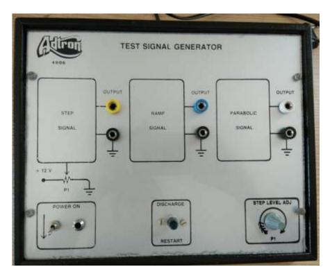
It is a complete instrument, required in the experiments of control engineering. It provides test signals of different waveforms and frequencies for feeding in as error signals. The input supply required is 230V, 50Hz AC. It gives very low frequencies (variable) step and Ramp waveform signals, which are essential for finding the response of various control circuits.
