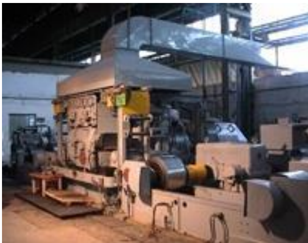
Photograph of Cold Rolling Mill
